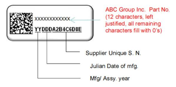
Standardized 2D Bar code format (QR or Data matrix) across all components and internal assemblies.
